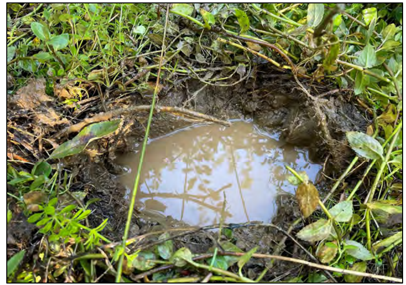
14. SP7 – saturation at the surface and inundation at 2” below the surface during the dry season indicate perennial wetland hydrology. October 27, 2023.
